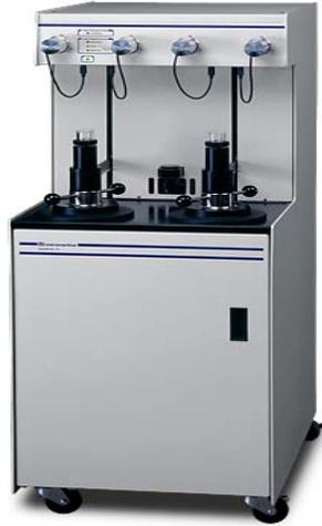
Figure 3.5: Micromeritics AutoPore III.
